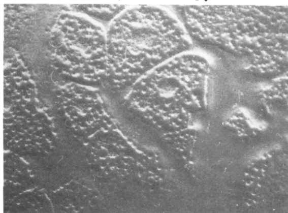
Figure 2. Enlarged view of the surface undulation pattern showing individual disklike islands and an ambiguous cellular organization of the islands.
